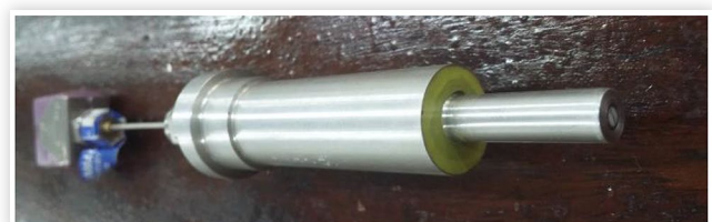
FIGURE 15 The erodible E-type thermocouple fitted in the machined Aluminum adaptor
